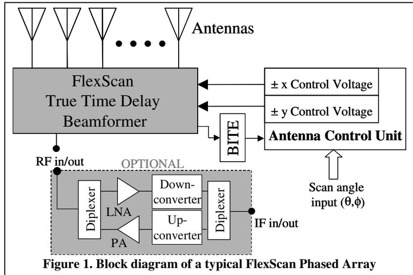
Figure 1. Block diagram of a typical FlexScan Phased Array
