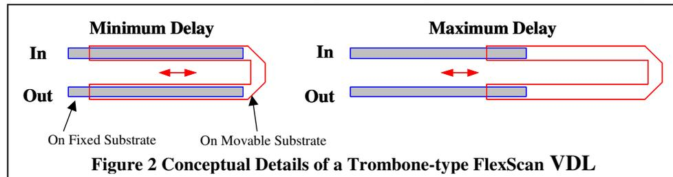
Figure 2 Conceptual Details of a Trombone-type FlexScan VDL
