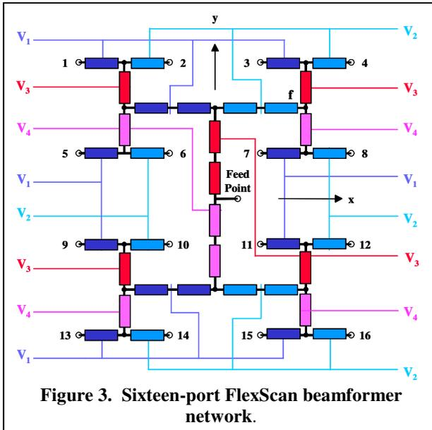
Figure 3. Sixteen-port FlexScan beamformer network.
