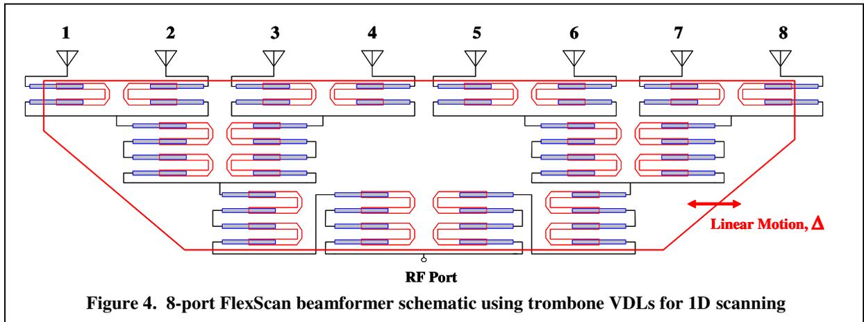
Figure 4. 8-port FlexScan beamformer schematic using trombone VDLs for 1D scanning
