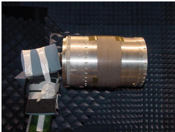
**Figure 5: 2 element high x 32 element roll prototype array**
